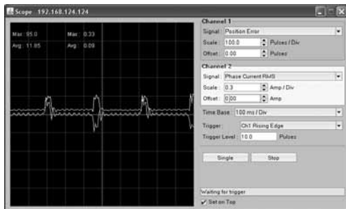
Minimal oscillation when motor positioned to target position.
