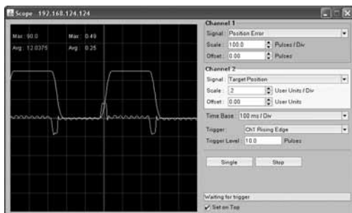
Position Error trace following the tuning of Position P-, I- and D-Gains
